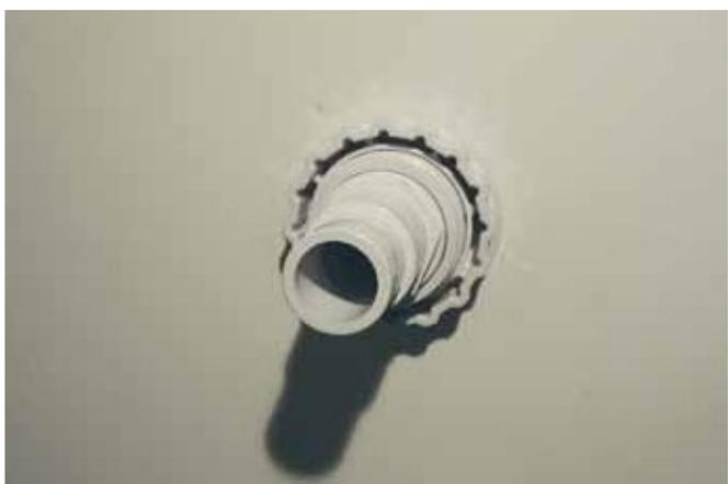
Make sure that the nozzle base does not twist, as this will cause wrinkles in the film!
