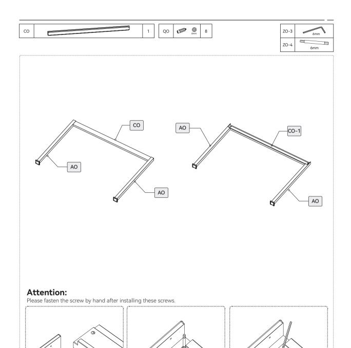
First, position the secondary beam, followed by the primary beam, taking care to note the motor connection cable on the primary beam. Then, connect the motor cable from the controller to the motor.
