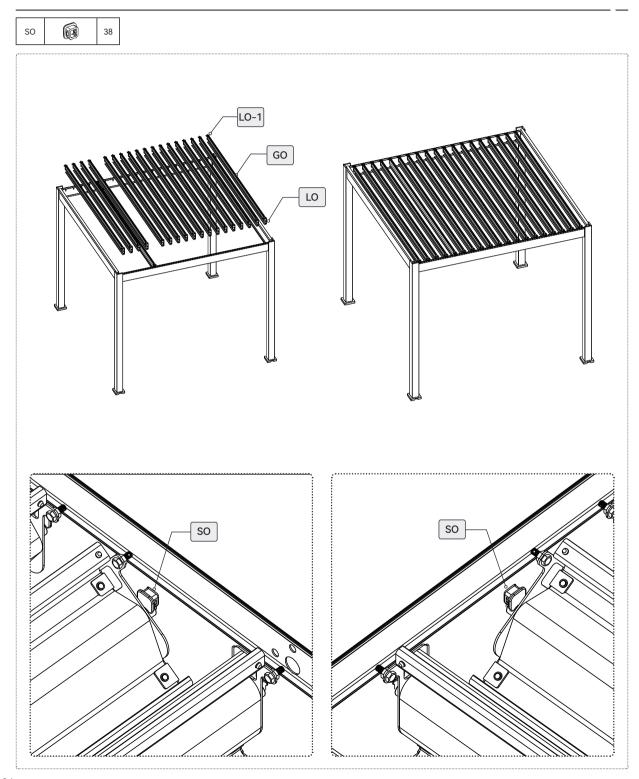
Attach the connecting rod to the side of the spindle louvre.
