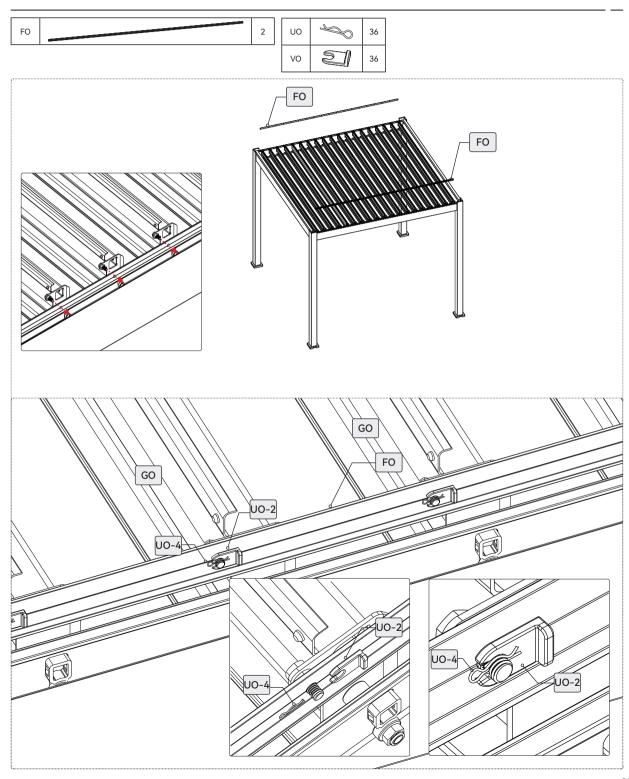
the corner aluminum is connected to the main shaft louver using lock nuts and washers.
