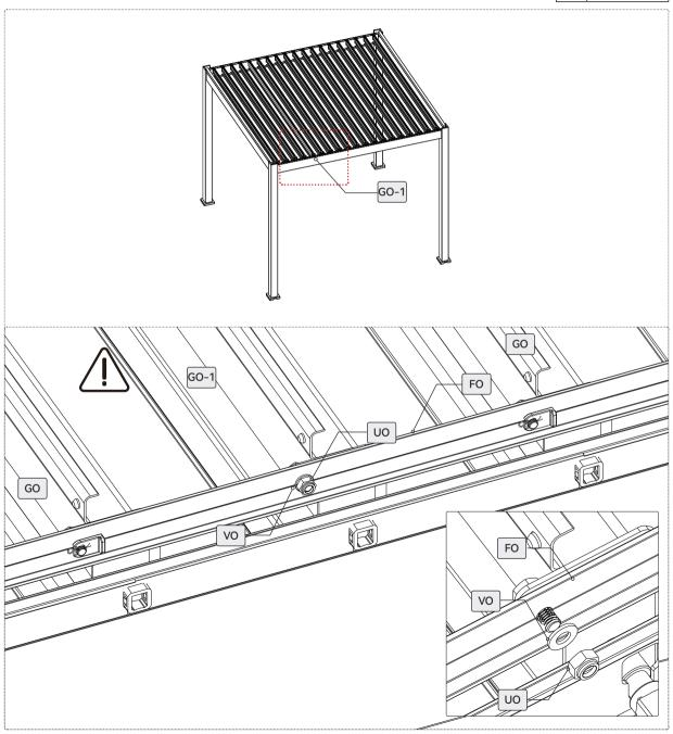
nstall the end cap onto the beam and secure the mounting holes with plastic covers.
