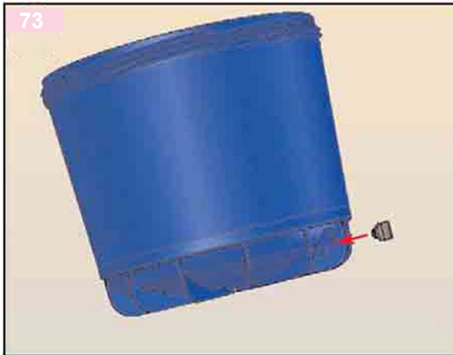
Check that the drain plug and o-ring are in position. Hand tighten only.
